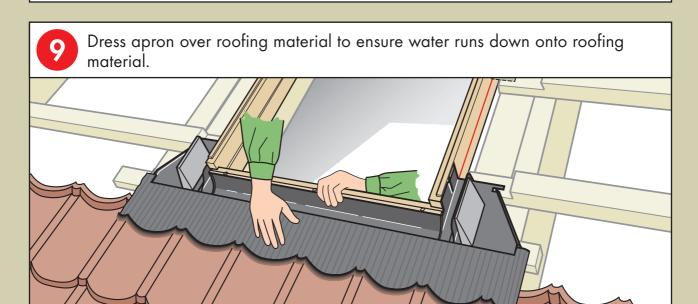
After fitting the apron to the roofing material, give the apron a "down bend" as shown - This will ensure the apron lays tight against the roofing material.
